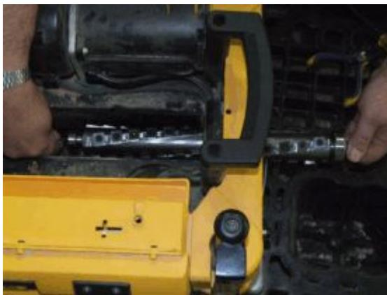
26. Carefully tap the head into position making sure the bearings are fully seated in the housings.
