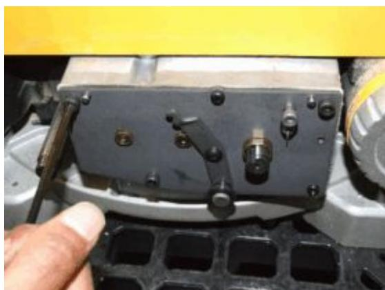
20. Pull the gear box back but DON'T completely disconnect it from the machine.
