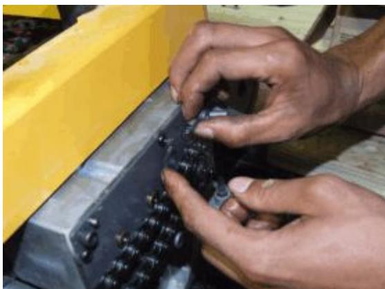
17. Remove the chain and sprockets together.
