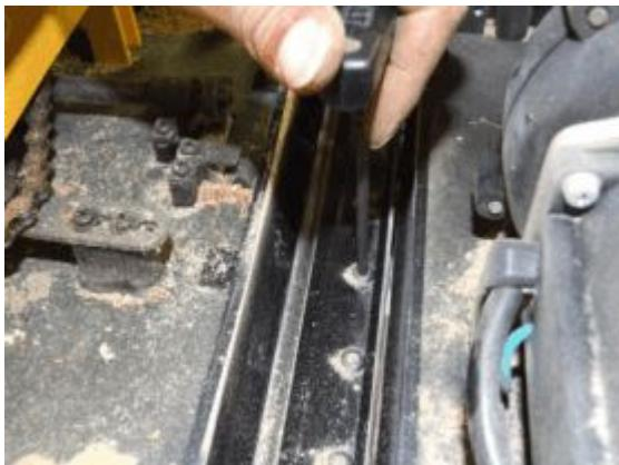
4. Remove the cutter rotate lock plate by removing the two Phillips head screws. Be careful to catch the spring that is underneath the bracket. Be careful not to strip out the screw heads as they are held in place with blue thread lock.
