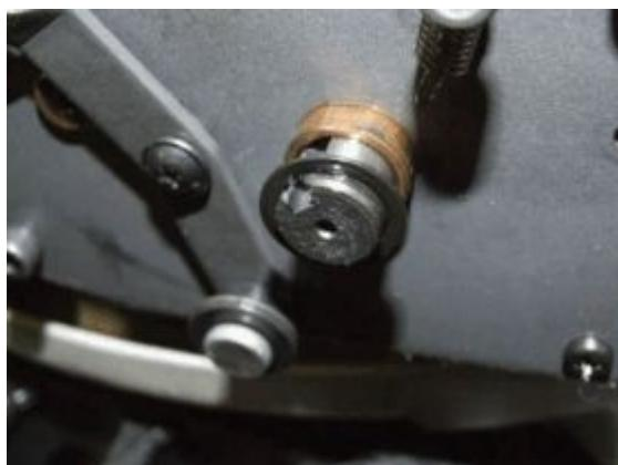
19. Remove the 3 socket head screws that hold the gear box in place.
