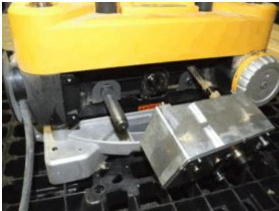
21. From the side opposite of where the pulley was, tap the head out using a piece of hardwood.
