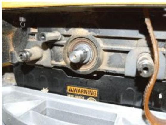
13. Remove the snap ring from inside the bearing housing.
