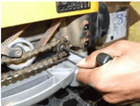
9. Remove the chain and sprockets together.
