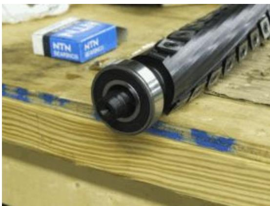
25. Carefully slide the new head through the bearing housing. Be careful of alignment so as not to bind the carbide knives and chip or break them. You can wrap the new cutterhead with blue painter's tape to help protect the carbide knives.
