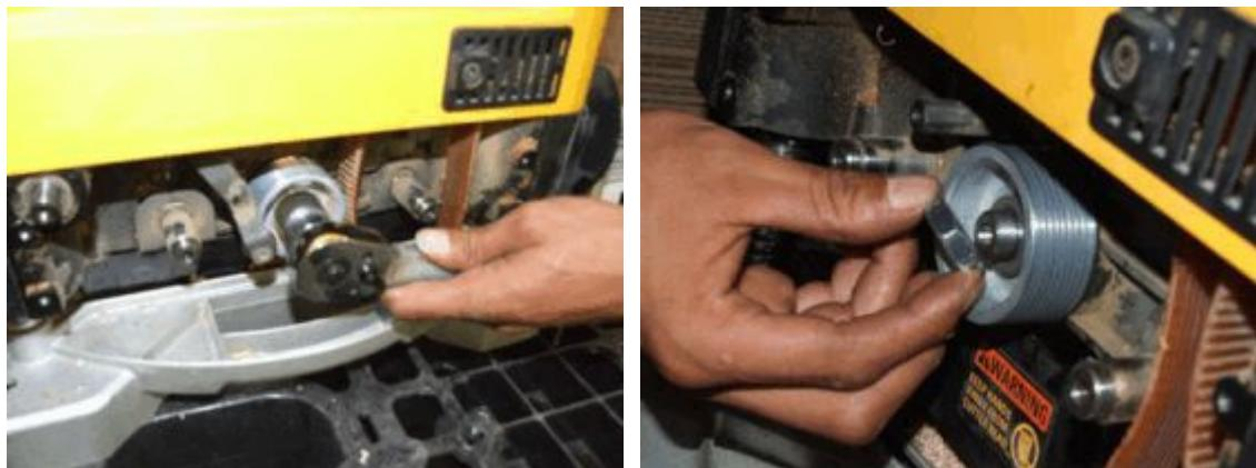
12. Slide the pulley off taking care not to lose the key, and remove the bushing from the shaft.
