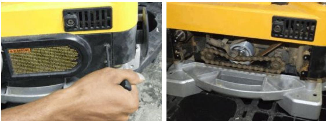
7. Unhook the tension spring and remove the idler arm, being careful not to strip the Phillips head screw which is held in place with blue thread lock.
